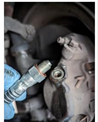
New hose and copper washer to attach to caliper.
