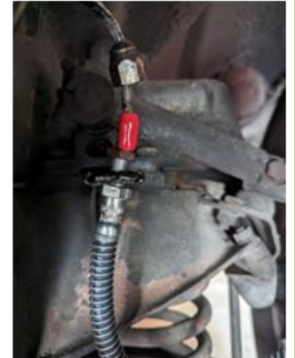
New hose loose in mount ready for hard line reconnection.
