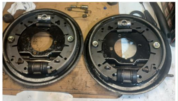
After new shoes and new wheel cylinders
