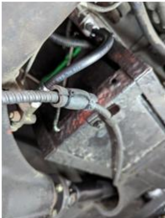
Hose added around hand brake case to prevent rubbing.
