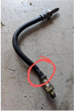
Rear hose with damage highlighted.
