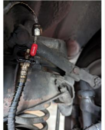
Hose loose in mount with hard line removed and capped.
