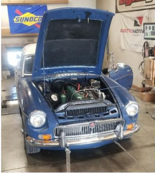
Figure 2: MGC Strapped on Dynamometer
